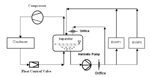
Overfeeding also ensures that the vapours coming out of the evaporator are at close to saturated condition without any superheat thus lowering compressor inlet gas temperature, which also means corresponding lower discharge gas temperatures, which are critical factor for ammonia systems working at low temperature applications. Higher discharge temperatures pose many problems for compressor.
